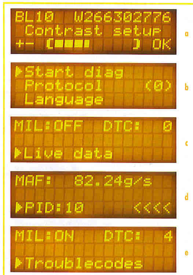
Figure 9. Displays: (a) Contrast setting, (b) Start menu, (c) Status display, (d) MIL/DTC PID Menu, (e) DTC trouble code numbers.
